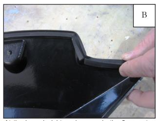
At the inward, right angle curve in the flare, cut a notch in the edge trim so when you along the part, the edge trim doesn't stretch.
