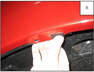
Install Tab (MT1-0014) over existing factory hole. There are two holes at the top center location. Refer to step 7 for proper hole for installation.
