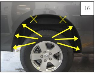
Remove these six factory installed screws using an 8mm socket wrench. Keep screws for installation of the rear flare. X's indicate a factory screw that will not be removed.
