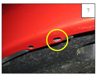
At location in step 6, there is a lip with two factory holes. One hole is a circle and one is an oval. The Tab (MT1-0014) and Clip (CL1-0022) will be installed over the oval. The oval is the hole more toward the front of the vehicle.
