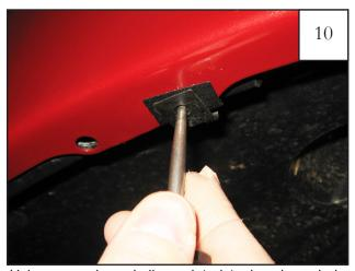
Using an awl or similar pointed tool, poke a hole through Tab (MT1-0014) using the Clip (CL1-0022) hole as a guide.
