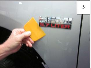
(OPTIONAL) If an emblem interferes with proper installation of flare, remove it. Apply adhesive remover to the emblem for ease of removal. Using a plastic putty knife, carefully remove it, taking caution not to scratch the paint.
