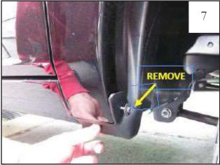
**2011-12 Models Only (Optional):** If you encounter a fit problem, remove inner piece at bottom rear of wheel well. Remove screws using an 8mm socket
