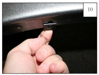
Install Clip (CL1-0022) over existing factory holes. There are two holes at the top center location. The hole for proper installation is the one toward the front of the vehicle. *NOTE:* The clip may fit over the lip loosely. This can be fixed by pinching the clip more tightly to the vehicle.
