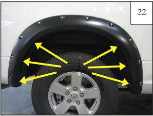
Hold flare in place start six supplied screws using an Phillips Head Screwdriver. *Do not tighten*.
