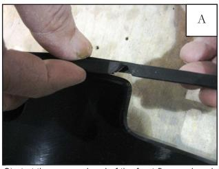
Start at the rearward end of the front flare and work toward the front. At the outward, right angle curve in the flare, cut a V out of the edge trim so when you wrap around the part, the edge trim doesn't bulge.
