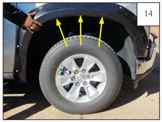
Hold flare to vehicle and re-install (3) factory screws (removed in Step 7) with a T15 bit. *Do not tighten*.
