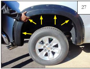
Hold flare to vehicle and install (5) supplied phillips head screws (SW1-0058) at each Clip location. *Do not tighten.* (If needed use an awl to align flare mounting holes.)
