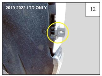
Install supplied Tab (MT1-0017) over the front location marked in Step 9. Install a clip assembly as indicated, on top of the Tab. See Step 13 for detail of clip attachment.
