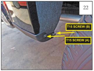
Locate the mud flap behind the rear wheel. Remove (2) factory installed T15 screws. NOTE: T15 screw labeled (B) will be re-used.
