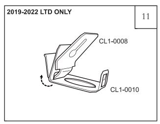
**NOTE: STEPS 11-13 APPLY TO 2019-2022 LTD ONLY.** Assemble Clip CL1-008 with CL1-0010 as indicated in the above diagram. Insert tab of CL1-0008 through slot in CL1-0010.
