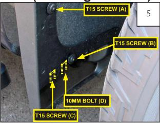
Remove (3) factory installed T15 screws, and (1) factory installed 10mm bolt. Note that two T15 screws labeled (A) and (B) above will be re-used to install the flare. You may discard (C) and (D).
