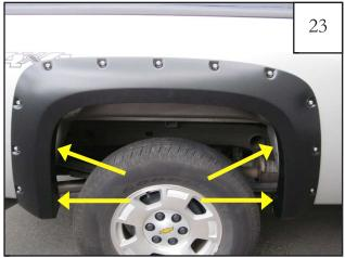
Start a supplied Screw (SW1-0050) through each of the remaining holes and into each Clip (CL1-0005) installed in step 21. If needed, use awl to locate holes.
