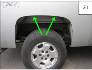
Slide a supplied Clip (CL1-0022) over top two factory holes. Clips may need to be adjusted to align with holes in flare. Note: Some vehicles with inner splash sheild will need to remove factory fasteners in indicated locations before installing the clips.
