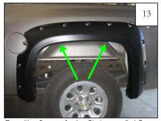
Reposition flare on fender. Start a supplied Screw (SW1-0058) through upper two hole locations and through each Clip (CL1-0022) installed in step 11. If needed, use awl to locate holes.
