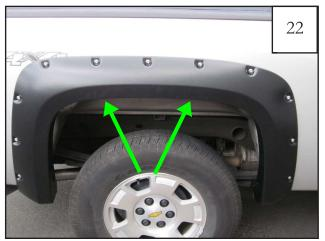
Reposition flare on fender. Start a supplied Screw (SW1-0058) through upper two hole locations and through each Clip (CL1-0022) installed in step 20. If needed, use awl to locate holes.
