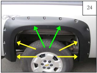
Fully tighten all screws starting with the newly installed Screws (SW1-0058) in upper two hole locations while pressing in on flare to ensure it is snug against sheet metal.
