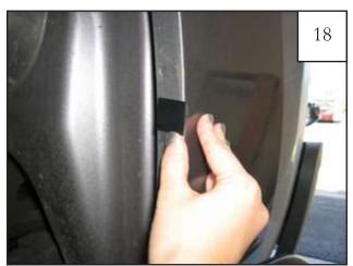
Center a supplied Tab (MT1-0002) over the marks made in step 16, aligning edge of tab with inside edge of fender lip (tab may extend over outside of fender).
