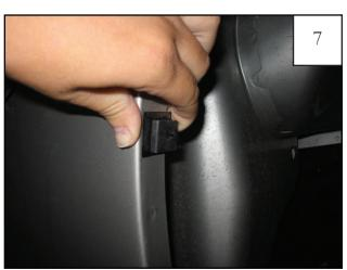
Slide a supplied clip over each black tab. Clips may need to be adjusted to align with holes in flare.
