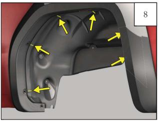
While holding the rear flare in place, mark the flare's (6) hole locations using a grease pencil. Remove flare after marking.
