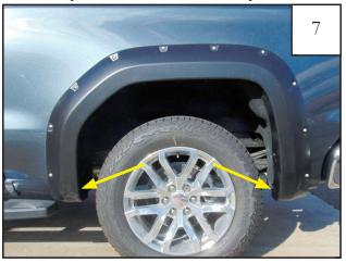
Loosely attach flare using (2) screws removed in previous step.
