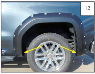
Loosely attach flare with factory screws removed previously.
