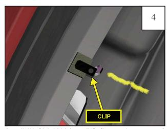
Install (6) CL1-0009 long "U" clips on the center of the foam tabs.
