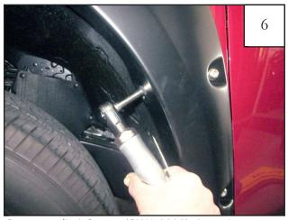
Start supplied Screw (SW1-0036) through top rear hole in flare and into factory hole in rear of wheel well. *Do not tighten.*
