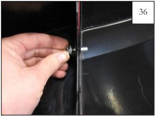
Align the holes in the Rear Main Flare with the holes in the Rear Bumper Piece, slide Screw/Washer assembly through (2 places).
