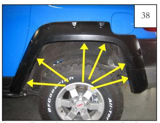
Position Flare on fender. Install six supplied Screws (SW1-0036). Do not tighten. NOTE: It is helpful to install one of the top Screws first.
