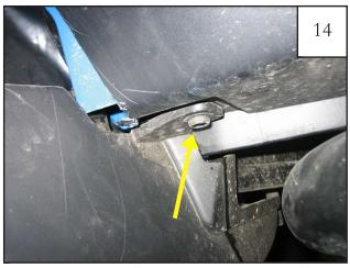
Remove third mud flap bolt, and remove mud flap.
