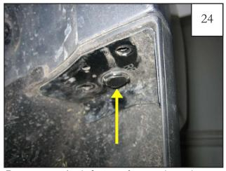
Remove one plastic fastener from mud guard.
