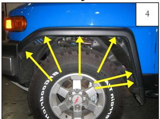
Remove six bolts from wheel well using a 10mm socket.
