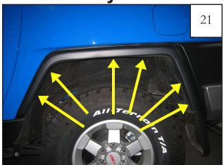
Using a 10mm socket, remove six bolts.
