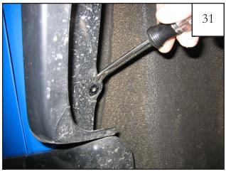
At front of wheel well, use pry tool or knife to pry plastic grommet from sheet metal. Discard grommet, leaving a square hole.
