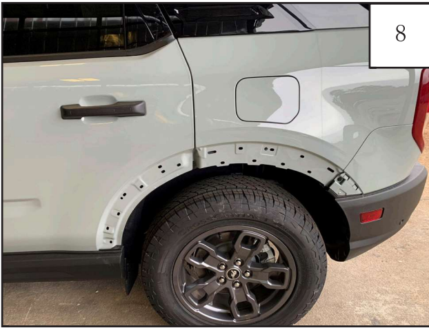
Remove factory wheel arch molding.
