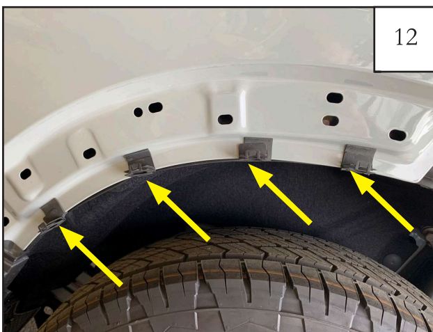
Install (4) CL1-008 and 4 CL1-0010 Clips over the foam pads
