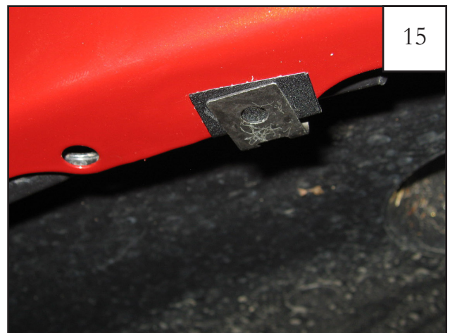
Install #10 U-Clip over 1"x1.5" Black Tab.
