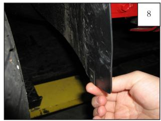
Slide a supplied "U" Clip onto factory hole in Splash Guard.
