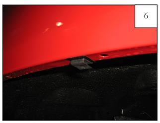
Slide the supplied "S" Clips over the Plastic Tabs on the fender lip (3 places).
