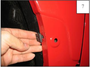
Slide two supplied "S" Clips over factory holes located in rear of wheel well as shown.
