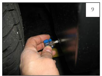
Hold the flare on the fender. Start a supplied #8 Truss-Head Screw through the lower rear hole in the flare and into the "U" Clip installed in Step 8.
