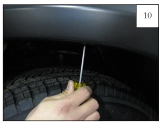
Use an awl if necessary to locate and align holes in flare and clips.
