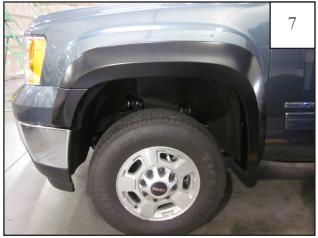
**OPTIONAL BUMPER PIECE:** Completed front flare installation.
