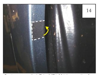
Center a supplied Tab (MT1-0014) over the four marks made in Step 12, aligning edge of Tab with outside edge of fender lip. Fold around back edge of fender lip and press firmly to adhere.
