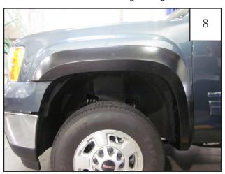
Completed front flare installation without bumper piece.
