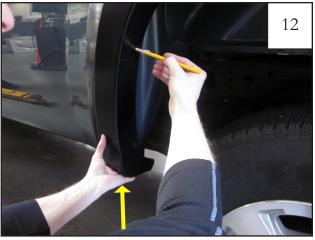
Pushing upward on the flare to ensure proper positioning, use a grease pencil to mark four hole locations. Remove screws installed in Step 11 and remove flare.
