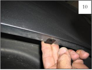
Center a supplied Clip (CL1-0022) over the two holes in Step 9. Clips may need to be adjusted to align with holes in flare. *Note: The raised collar on the Clip should face upward into the interior of the fender.*
