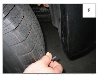
Install three supplied Plastic Push Retainers in remaining holes in flare.
