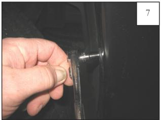
Holding flare in position on fender, reinstall factory screws removed in Step 7.
