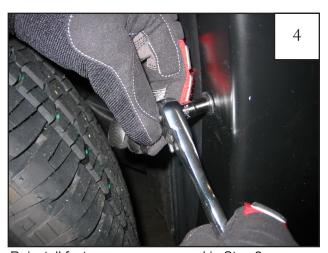
Reinstall factory screws removed in Step 2.
