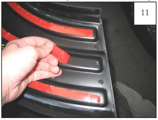
Peel the red liner entirely from the CENTER tape pad. Peel 2" of liner from each of the other two tape pads, folding out to form tabs.
