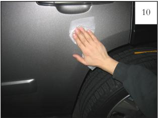
Using a supplied alcohol wipe, clean the area where the door piece will be installed. Make sure area is dry before starting installation.
