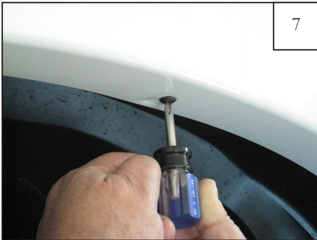
Start a supplied Screw (SW1-0050) through topmost hole in flare and into Clip (CL1-0005) installed in Step 5. Do not tighten.
