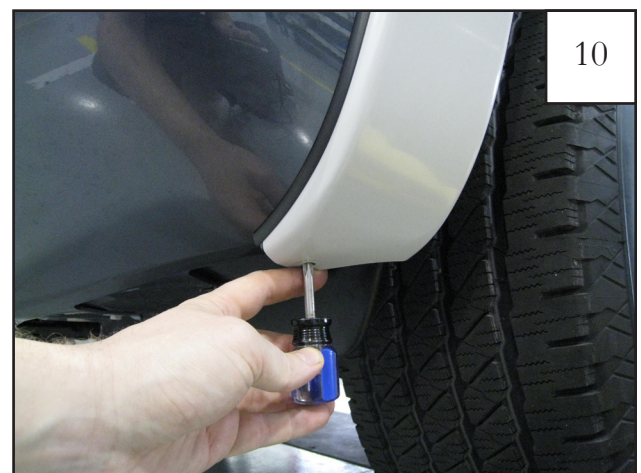
Start a supplied Screw (SW1-0050) through flare and into Clip (CL1-0005) installed in Step 9. Do not tighten.
