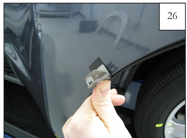
Open the door, and slide four supplied Door Clips over door lip, centering on Black Tabs.
