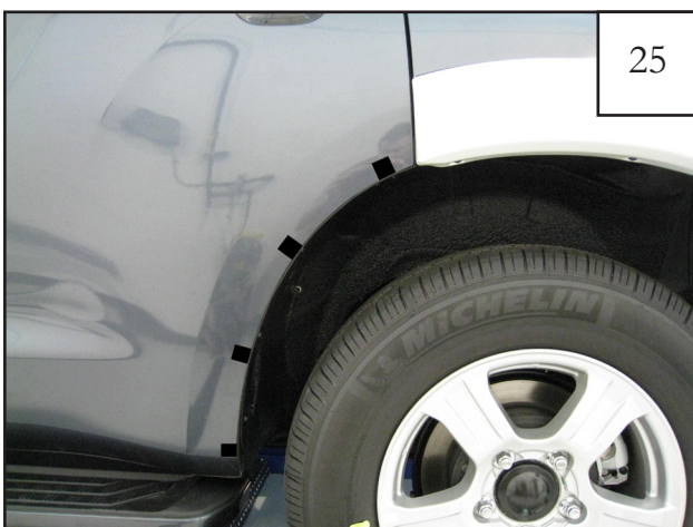
Center four supplied Black Tabs (MT1-0002) on marks made.
