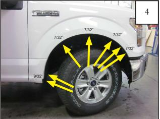
Remove five factory screws with a 7/32" socket wrench. Remove two rear most factory screws with 9/32" socket wrench. Save screws for reinstallation. **Note:** If you have factory flares you will need to remove them to install Husky flares.
