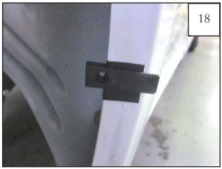
Install a Clip (CL1-0009) over each of the four Tabs (MT1-0034) placed over the upper 4 marks made in Step 16.
