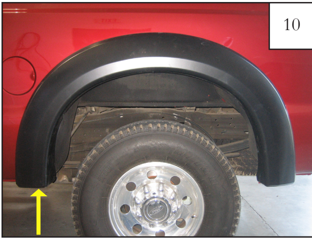
Reinstall bolt removed in Step 4 with a 10 mm socket.
