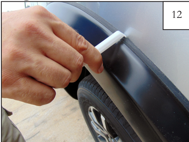
Using supplied Edge Trim Tool, seat edge trim against vehicle by hooking curved end under edge trim at one end of flare. Next, slide around outer edge of flare to the other end.
